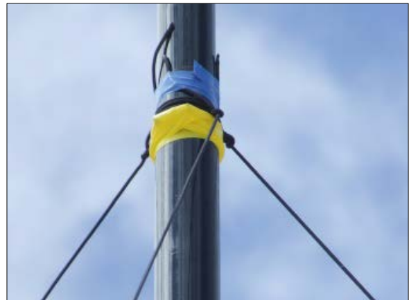
Fig. 41 Attachment of the guy lines (Photo: Lagunaria DX Group)
