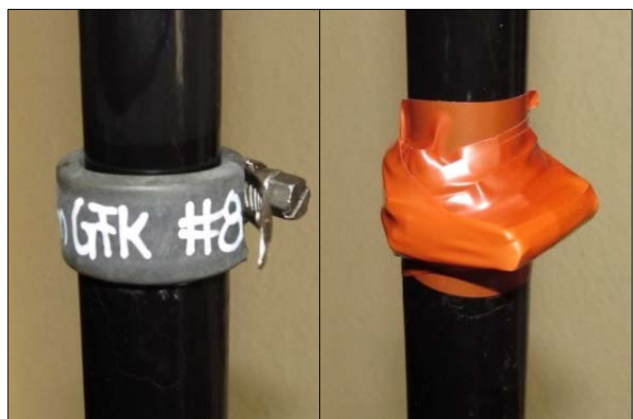
Fig. 39 Mounted clamp (left) and wrapped with adhesive tape (right) (Photo: Lagunaria DX Group)
