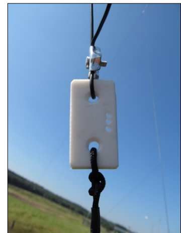
Fig. 28 Insulator made of PTFE (Photo: Lagunaria DX Group)
