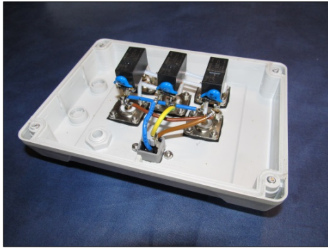
Fig. 37 Interior of the VDA switch box (Photo: Lagunaria DX Group)
