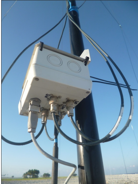
Fig. 42 Completely wired VDA switch box (Photo: Lagunaria DX Group)
